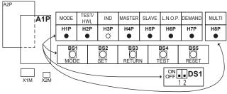
DIP switches DS<sub>1</sub> BS1~BS5 Push buttons H1P~H7P 7-LEDs display
