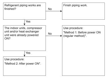
It is very important that all refrigerant piping work is done before the units (compressor unit, heat exchanger unit or indoor units) are powered on.
